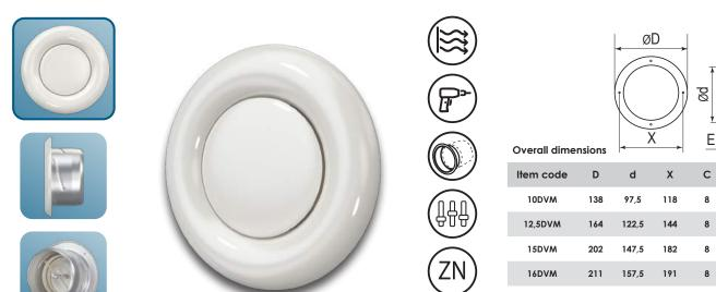
DVM is designed for exhaust ventilation systems and mounted into walls or dropped ceilings. Made of steel with polymer coating and can be installed in premises with high temperature environment. Mounted with round ventilation ducts via flange.
