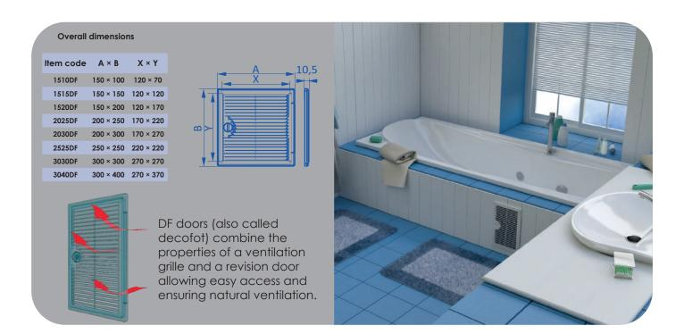
Decofot is applied onto wall or other surfaces and not intended for an in-hole installation. So, the device suits for mounting holes with wavy edges. The only demand is the access door being bigger than the mounting hole size. When mounting the device above the eye level, "shutters up" installation is recommended to hide the mounting hole. When mounting the device below the eye level, "shutters down" installation is preferable.
