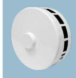
Mounted with round ventilation ducts of 100-125 mm in diameter and used for filtering the air intake. The device also allows to adjust the airflow capacity up to complete cutting the intake off. Adjustment is done by rotating the head. Used in SAV supply valves.
