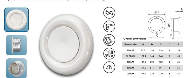
DUM is made of steel with polymer coating and designed for supply-exhaust ventilation systems and air-heating systems. Can also be installed in premises with high temperature environment. Mounted into walls or dropped ceilings. Airflow is controlled by rotating the valve part.
